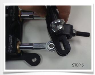
5. NOW SLIDE THE LOWER ROD END BACK INTO ITS SLOT IN THE PIVOT BLOCK. THE PIN GOES IN FROM THE TOP SIDE WITH TWO WASHERS ON THE TOP AND ONE WASHER AND A COTTER PIN ON THE BOTTOM. BEND THE COTTER PIN ALL THE WAY AROUND SO THAT IT WILL NOT FALL OUT OR INTERFERE WITH ANY MOUNTING BOLTS, STRAPS, LOOSE CLOTHING ETC.. HOLD THE TOP OF THE PIN WITH A PAIR OF PLIERS IF NEEDED TO ASSIST IN PROPER BENDING OF THE COTTER PIN.
